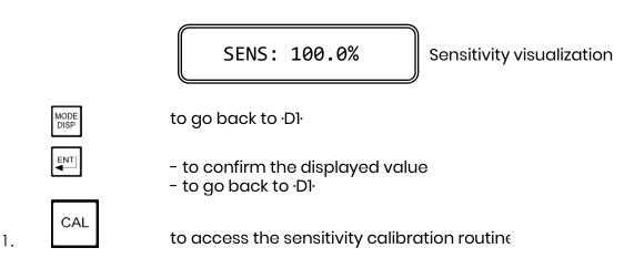
The sensitivity calibration is suggested when the readout is lower/higher compared with the DPD test. This adjustment must be effected when installing the flow cell and Chlorine or D.Ozone sensor after the stabilization of the readout.
