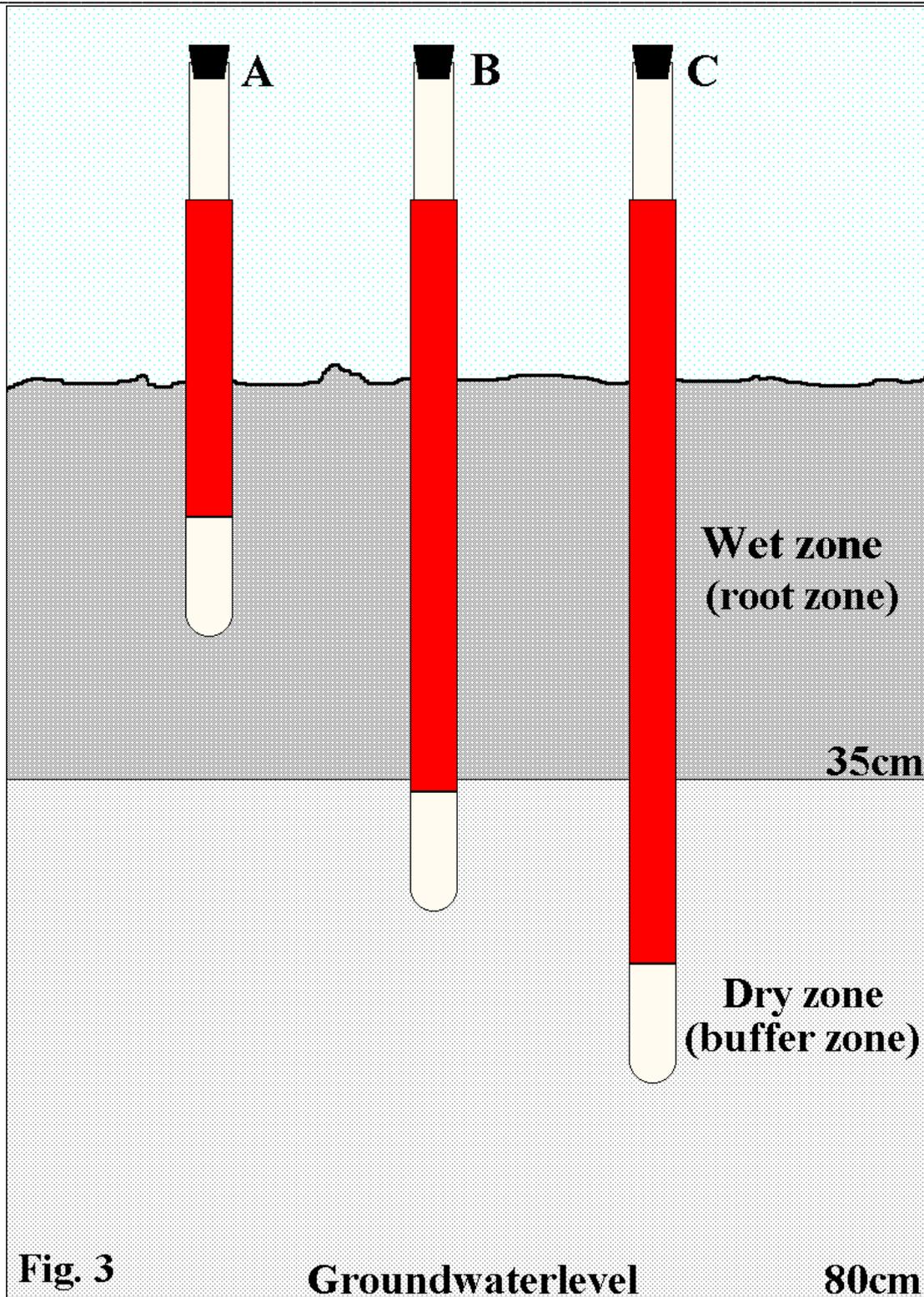
Tensiometer "A" is placed with the ceramic cup in the middle of the rootzone of the plants (in this case: 20cm).
