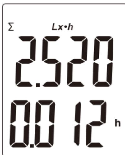
In integral interface, the upper half of the screen shows the integral of illumination in unit of  $Lx \cdot h$  or  $Fc \cdot h$ , the lower part shows the time span for integral, in unit of hour(h).
