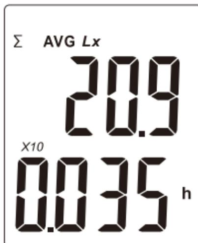
In average integral interface, the upper half of the screen shows the average illuminance in unit of  $Lx$  or  $Fc$ , the lower part shows the time for integration, in unit of hour (h).
