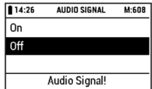
Select the desired memory space warning mode (On or OFF) using the [Up] and [Down] buttons.
