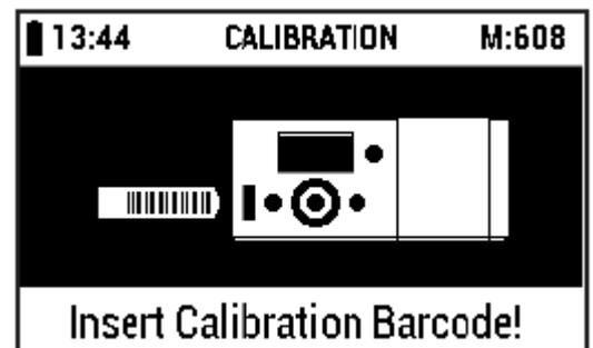
Remove the barcode strip for calibration from the pack (included in the scope of delivery of reflectometer). Insert the barcode all the way into the barcode reader in the direction of the arrow in a smooth motion from left to right, and then remove it again.
