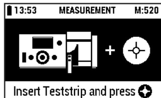
Insert the test strip into the test strip adapter and press the [START measurement] button.
