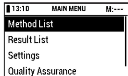
Pressing the [Up] and [Down] buttons takes the Reflectometer to the different submenus.
