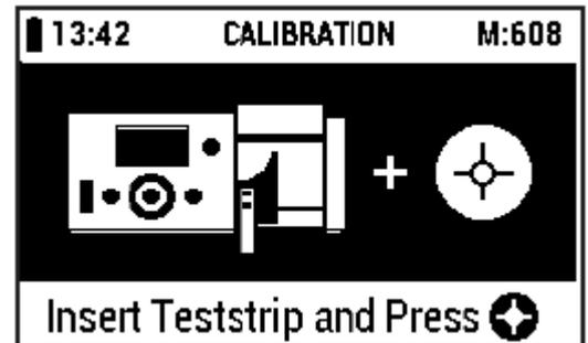
Insert the calibration strip of the recalibration set (included in the scope of delivery of reflectometer) into the strip adapter with the beveled edge outwards and upwards and press the [START measurement] button.
