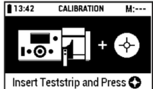
Insert the calibration strip of the recalibration set
