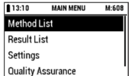
Press [START measurement] button to return to the last used method
