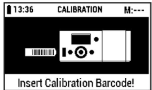
Remove the barcode strip for calibration from the pack (included in the scope of delivery of reflectometer). Insert the barcode all the way into the barcode reader in the direction of the arrow in a smooth motion from left to right, and then remove it again.
