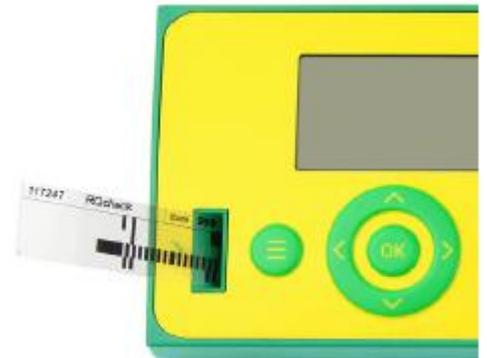
Insert the test strip for RQcheck into the test strip Adapter and press the [START measurement] button.
