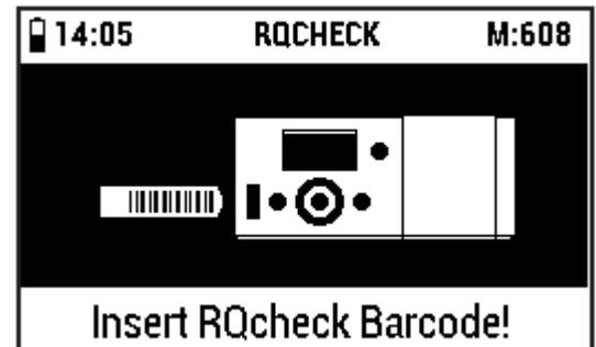
Remove the barcode strip for RQcheck from the pack. Insert the barcode all the way into the barcode reader in the direction of the arrow in a smooth motion from left to right, and then remove it again.
