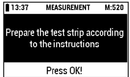
Immerse the test strip into the sample as described in the Reflectoquant® package insert (Reflectoquant® pack) and press the [OK] button.
