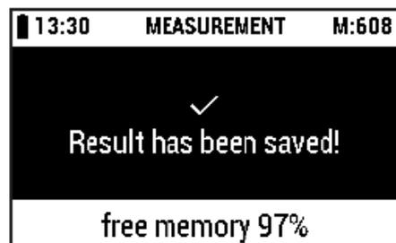
The save hint is shown only if memory space warning is on (see section 2.9.10, "**Setting the memory capacity warning**").
