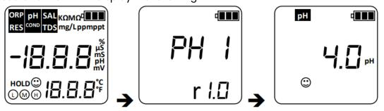
All segments ON -> model name + software release -> measurement
