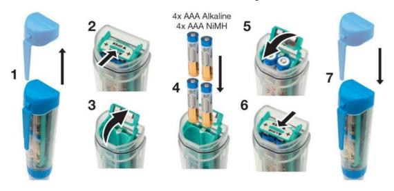
Make sure the batteries have correct polarity with positive pole upside.
