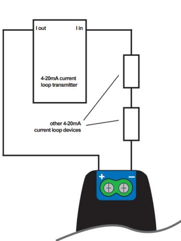
Connecting to a current loop transmitter.
