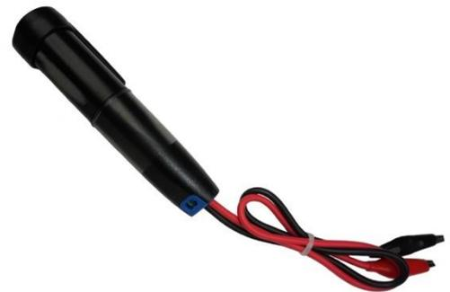
This stand-alone data logger measures and stores over 32,000 current loop readings over a 4-20mA d.c. range at a resolution of 0.05mA d.c.
