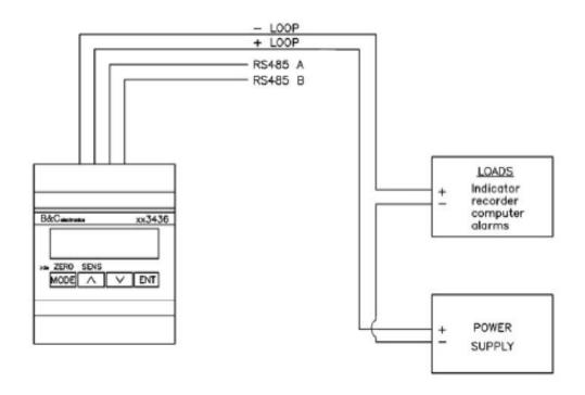
Connection to a PLC or data logger
