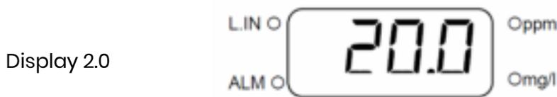
From this display it is possible the access to the calibration procedure of the temperature probe if this function is enabled by the operator.
