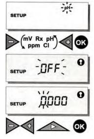
Pressing OK button, the display will show 0000. To set a password use (+ or-) buttons to increase or decrease value that composes the password. To shift from the first digit to the followings ones press Right Arrow. Press OK to confirm the password.
