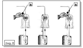
a normal syringe to suck liquid from the discharge nipple while the pump is in operation, continuing until you actually see the liquid rise in the syringe.
