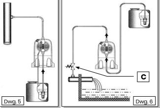
pump is shut down. If the problem persists, install a properly calibrate counter-pressure valve (C) between injection point and the valve. In the case of the liquids that generate aggressive vapors, do not install the pump above the storage tank unless the latter is hermetically sealed.
