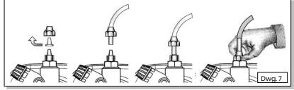
F Whenever the pump is dismantled from the pipework, you will be well advised to replace the caps on the connectors to avoid residual liquid being spilled. Before attaching the delivery hose to the plant, prime the metering pump by going through the sequences shown in (Dwg. 8). Before finalizing the installations of the discharge hose, make sure that the pump strokes will not cause it to move and bump into rigid bodies. In case of priming difficulties, use
