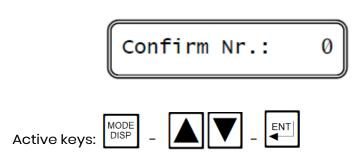
The double insertion of the new code assure the memorization of the right code, avoiding the insertion of two different access number.
