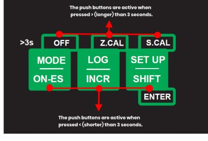
Push < 3 seconds 1. MODE / ON-ES 2. LOG / INCR 3. SET-UP / SHIFT Push > 3 seconds OFF Z.CAL S.CAL ENTER
