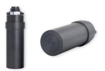
Technical Specifications (common to all probes)Measuring method: NephelometricResponse time: 10 sInternal sensor: for empty cell and dirty lens checkingPreamplifier: built-inPower: ± 12Vdc from TU 7685Ambient Temperature: 0/50 °CSample Temperature: 0/50 °CSample Pressure: 6 bar max. a 20 °CConnector: IP 67Optical window material: AcrilicPipe Tee for direct inline mounting: 2"(DN 50)Diameter: 40 mmCable length: 150 m max.
