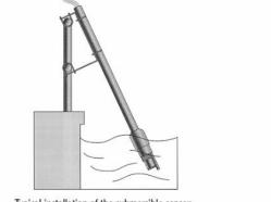
Typical installation of the submersible sensor.
