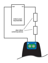
Connecting to a current loop transmitter.
