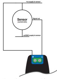
Connecting to a current source sensor.
