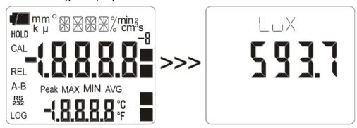
• AUTO/OFF: the AutoPowerOff function can be disabled by simultaneously pressing this key and the "HOLD" key when turning the instrument on.
