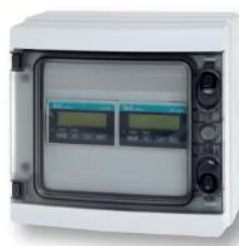
Enclosure for 2 transmitters Dimensions: 215x210x100 mm Protection: IP65 Wall mounting: with brackets, to be ordered separately
