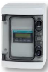
Enclosure for 1 transmitter Dimensions: 143x210x100 mm Protection: IP65 Wall mounting: with brackets, to be ordered separately
