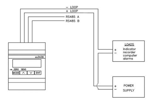
Connection to PLC or data logger
