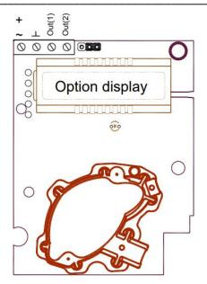
Figure 2. PCB with jumper to configure OUT2 for current output 4—20mA or voltage output 2—10VDC
