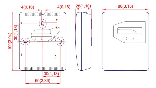
Figure 5. Sensor dimensions in mm and (inches)
