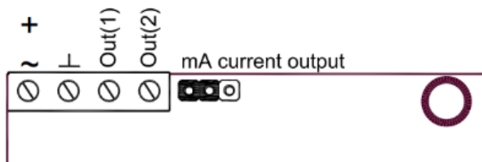
Figure 2. PCB with jumper to configure OUT2 for current output 4–20mA or voltage output 2–10VDC
