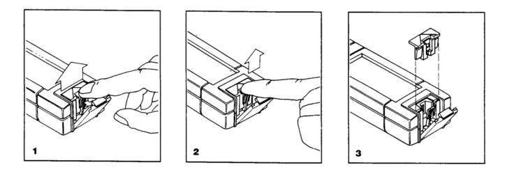
Very particular care must be taken if/when cleaning its small optical windows: never use a screwdriver or any other hard or sharp implement which might scratch or break these surfaces. Ensure that all surfaces are thoroughly dry before replacing the carrier.
