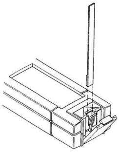
Reopen the hatch, and the display will revert to **CAL**. Remove the test strip, and check for reasons. This procedure must be repeated until **GO** is obtained.
