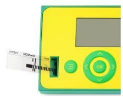
Insert the test strip for RQcheck into the test strip Adapter and press the [START measurement] button.
