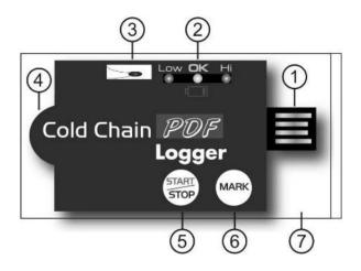
(1) USB2.0 plug & play connector. USB driver is not required.
