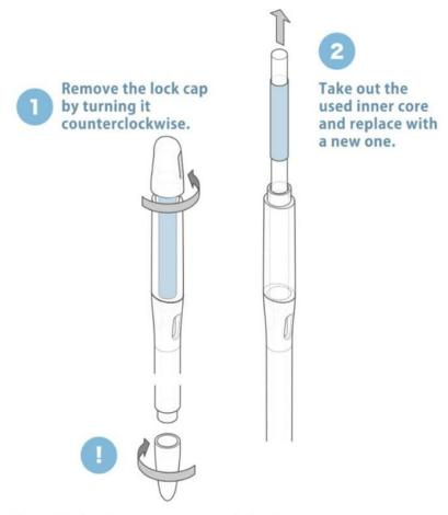
Open the bottom screw cap and check if any core material is left inside.
