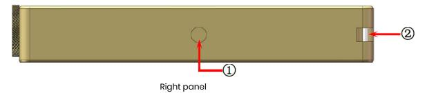
1)three foot mounting hole 2) wrist mounting groove
