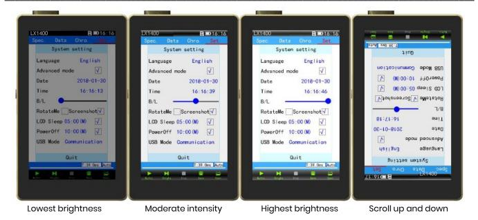
Left and right sliding brightness bar can adjust the brightness of the screen by figures
