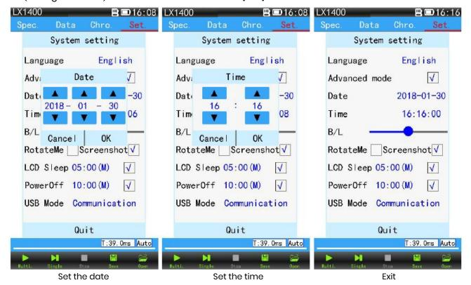
The screen brightness adjustment: Left and right sliding brightness bar can adjust the brightness of the screen, and then click [exit], adjust the completion (as shown below).
