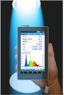
Press the "power button" or "stop" icon to stop the test
