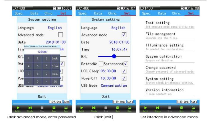
◆Set the date and time: After click "Date", pop up dialog box, click the up and down arrows to adjust the date to the correct date, click 【ok】; Use the same method to set the device time to the correct time (see figure below). After the end of the set click [exit]
