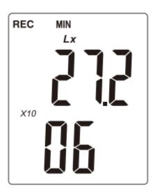
"MIN" at the top of screen means that the maximum storage groups in current manual storage area is up to 60; The upper part shows the current saved value of illumination, the lower part shows the current storage number of data.
